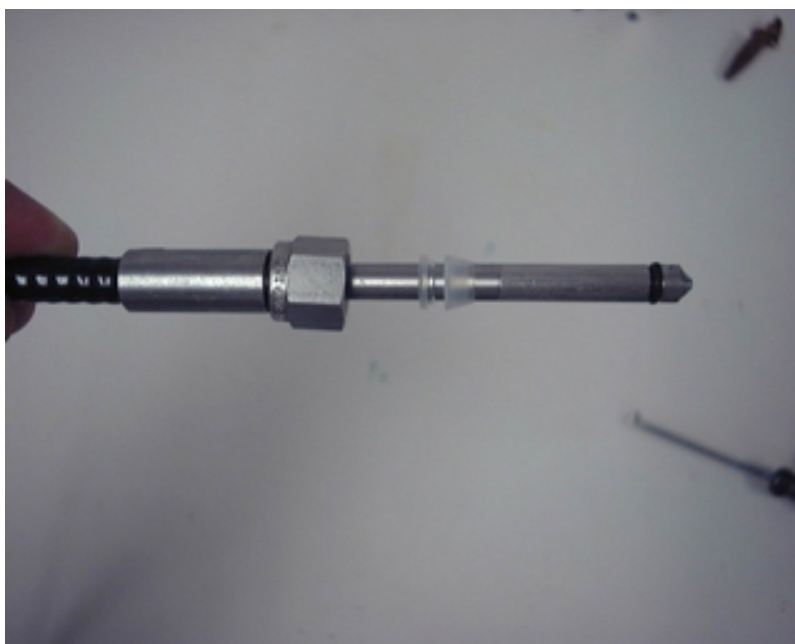
Figure 8. Properly assembled fiber terminator
