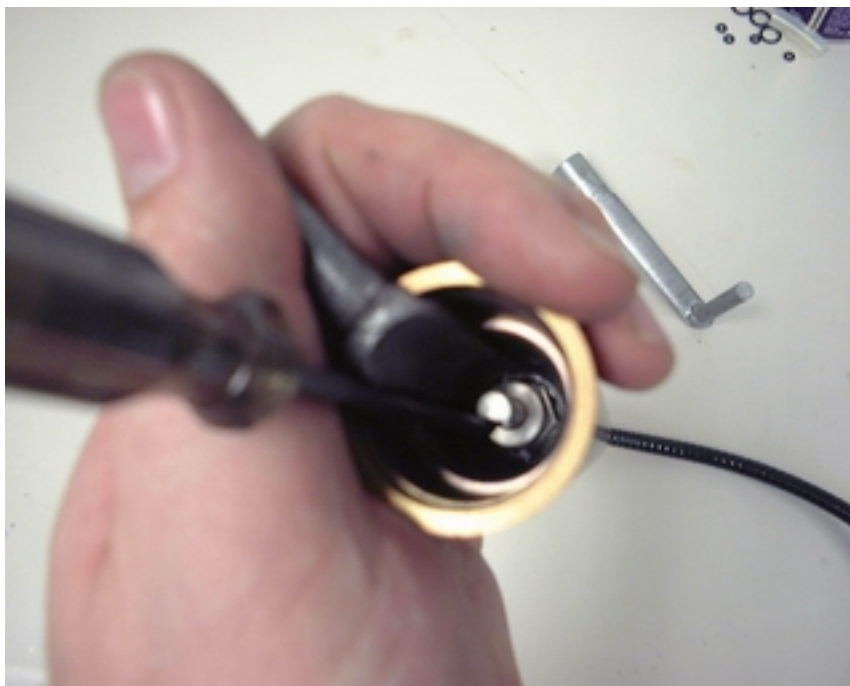
Figure 7. Holding the mirror shaft with pick to rotate (or hold) mirror.
