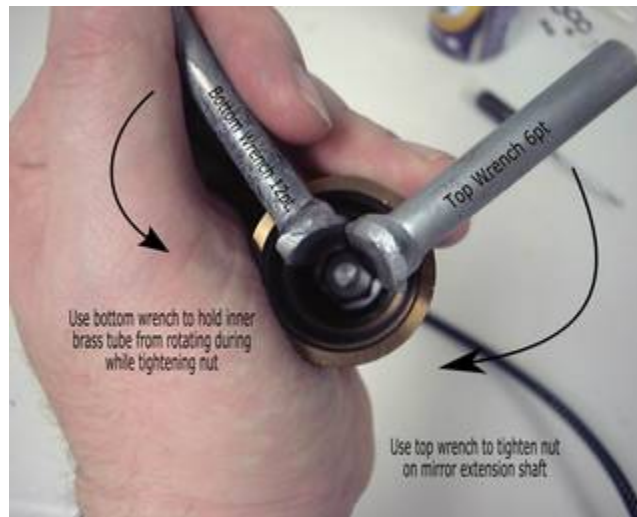
Figure 6. Proper wrench technique
