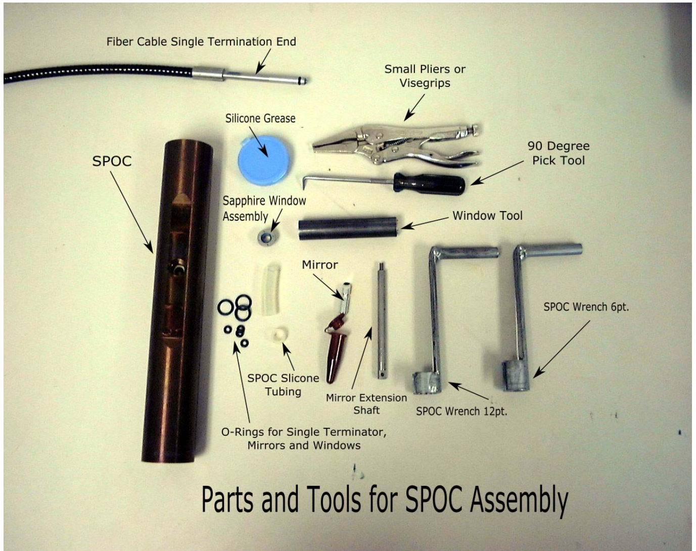
Figure 1. Parts and tools for SPOC assembly
