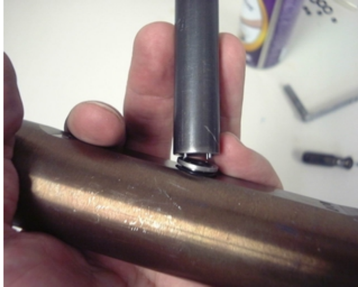
Figure 11. Carefully engage window with window tool
