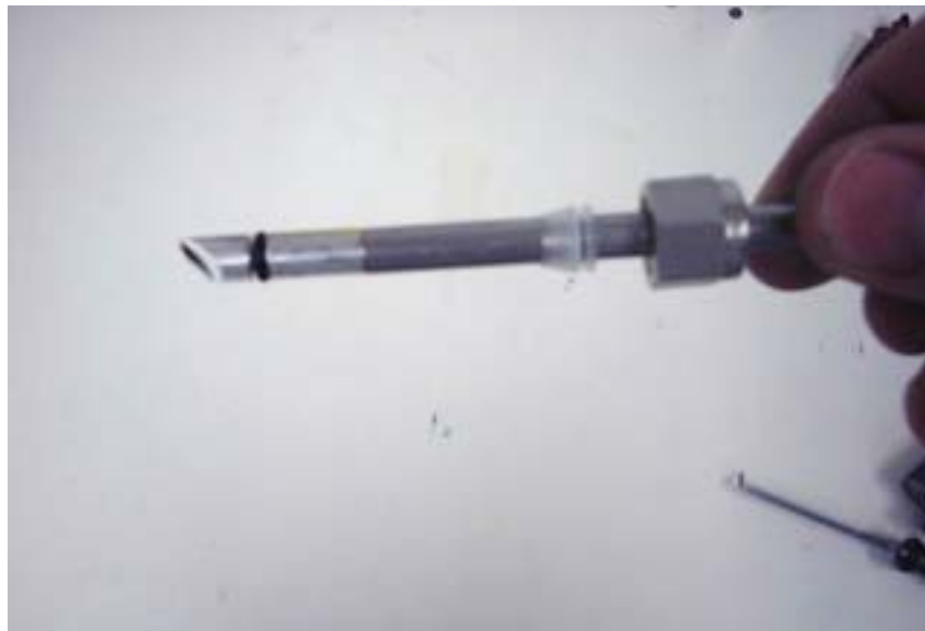
Figure 5. Properly constructed SPOC mirror assembly
