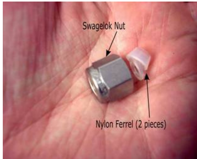
Figure 4. Swagelok nut and nylon ferrule (Note: ferrule is misspelled in photo)
