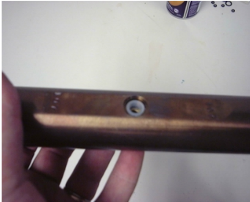
Figure 9. Window SPOC seal inserted
