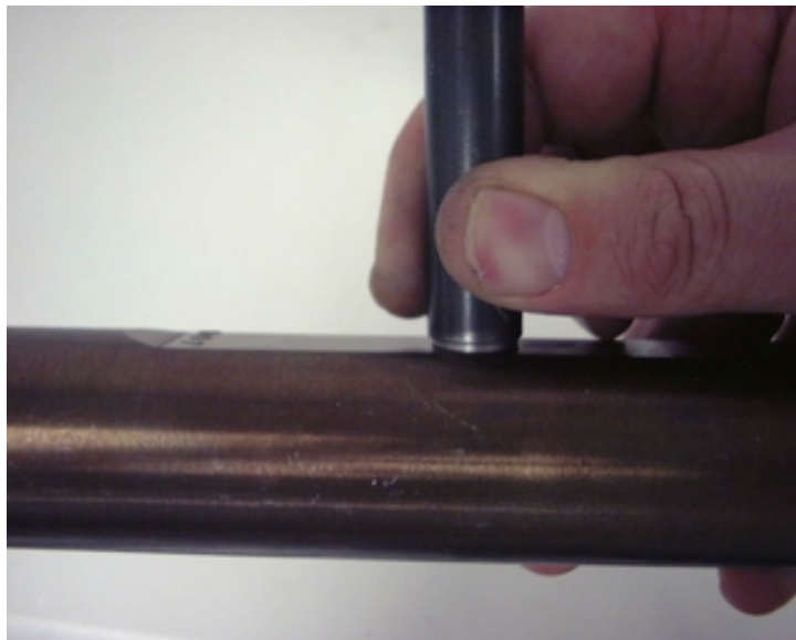
Figure 12. Fully seat tool's pins into window's holes
